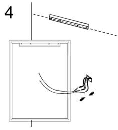
You may hardwire both cables to the same power supply. Connect the on/off switch to the white cable (Main) if one is used. A separate power supply is required for the Clock (black cable).
